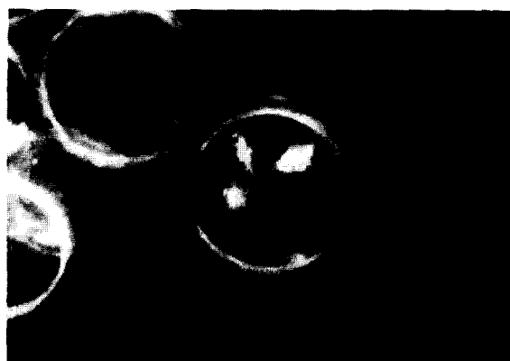
Figure 2 Optical photomicrograph (dark field) of \sim 200 \mu\text{m} polymerizing droplets withdrawn from a stirred reactor. Note the presence of floc inside the centre droplet
